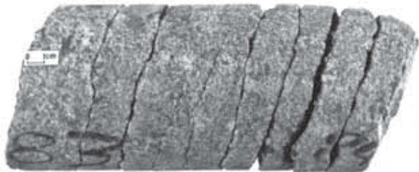
Figure 14 Non-symmetrical core discing (Stacey &Wesseloo, 2002).
