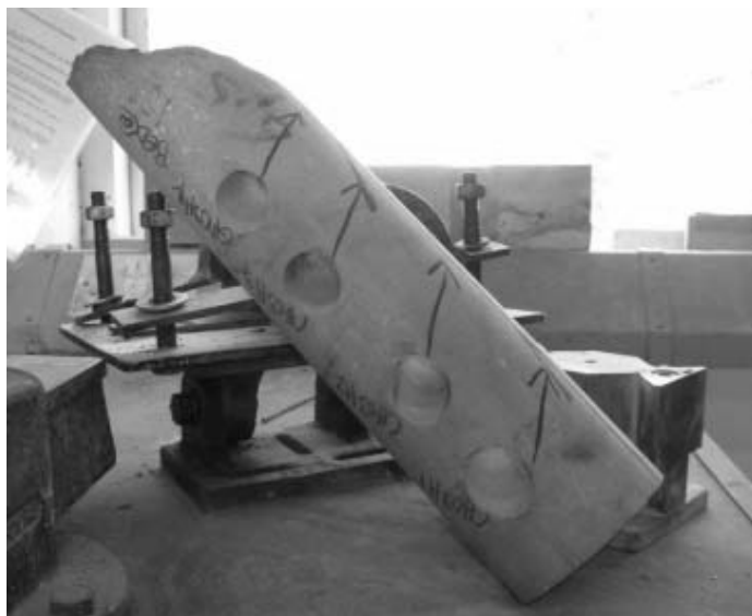
Figure 25: Acoustic emission sampling from an orientated 63mm
