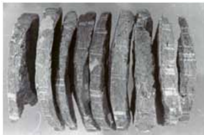
Figure 12: Symmetrical core discs (Stacey &Wesseloo, 2002).
