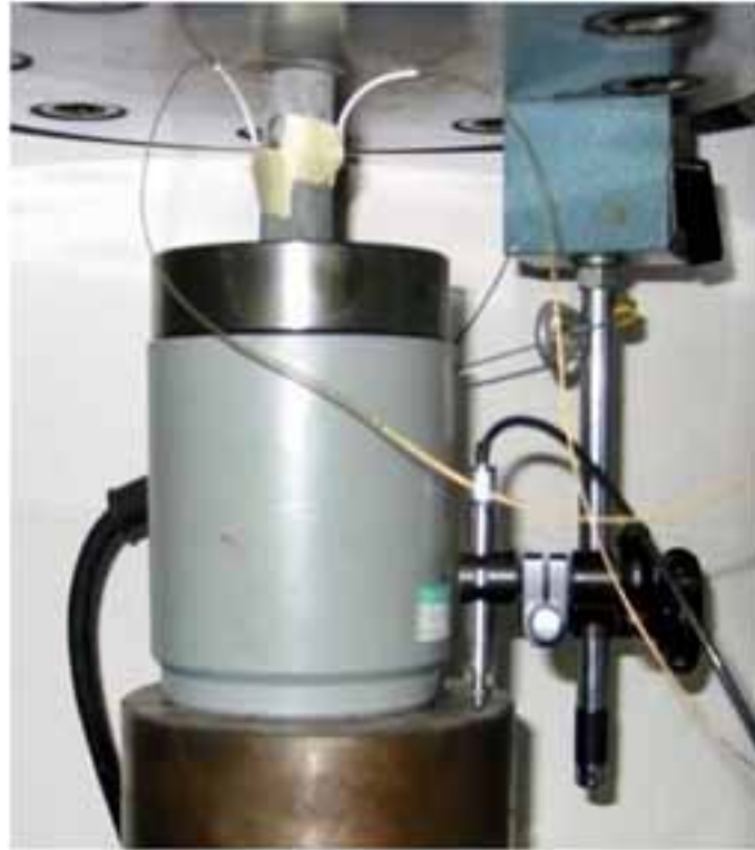
Figure 26: Test sample with acoustic emission sensors attached (Golder Associates)
