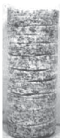
Figure 10: Borehole core with discing (Matsuki et al, 2004).
